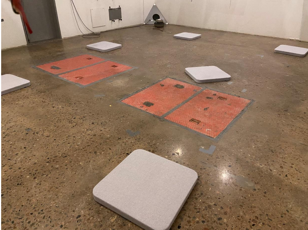
Picture 3 – kvadrat rundad 600x600mm, setup with 6 pcs mounted on the floor of the reverberation room.
