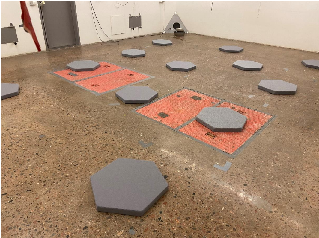
Picture 2 – Hexagon 600mm, setup with 12 pcs mounted on the floor of the reverberation room.
