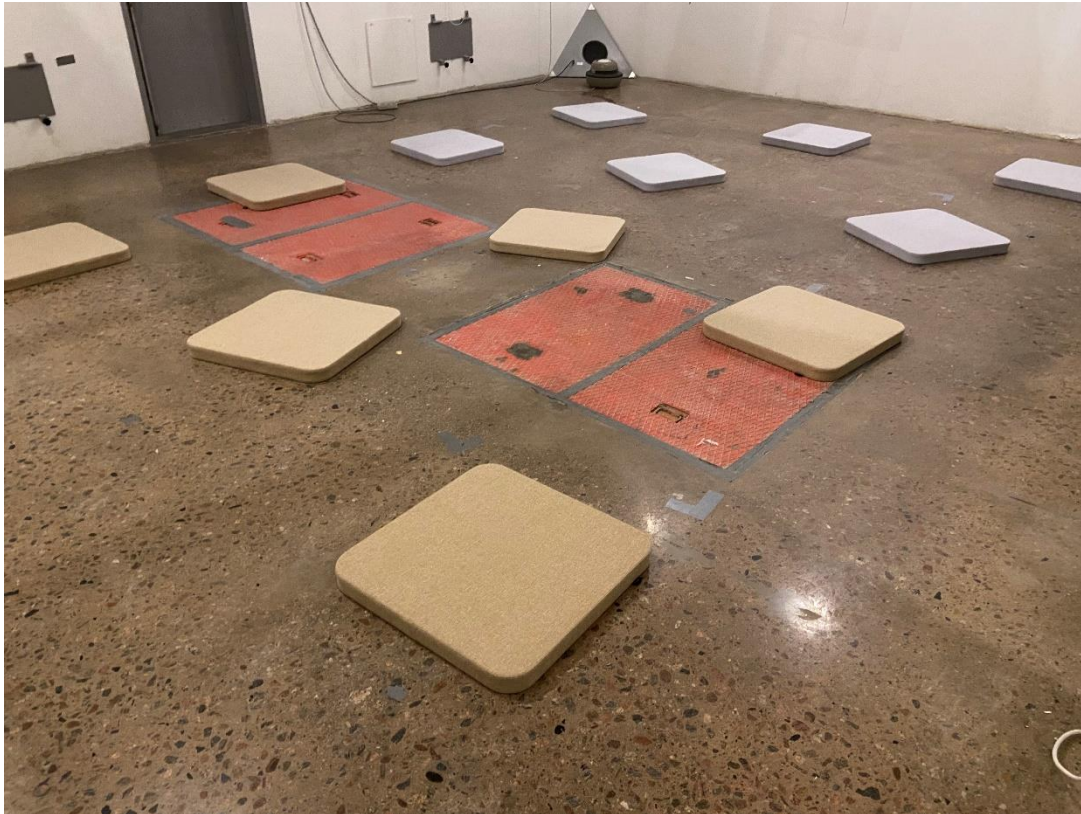
Picture 3 – kvadrat rundad 600x600mm, setup with 6 pcs mounted on the floor of the reverberation room.
