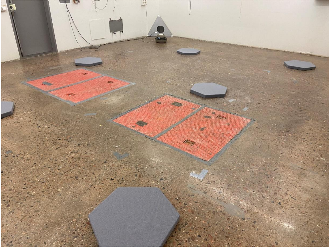
Picture 1 – Hexagon 600mm, setup with 6 pcs mounted on the floor of the reverberation room.
